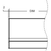
Note:- length dimensions are not including end caps. (2mm per cap will be added to total length)
